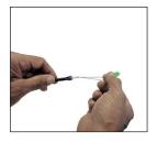
Step 4: Prepare the connector Clamp the fibres and remove the mesh backwards. Ready to connect to the adapters.
